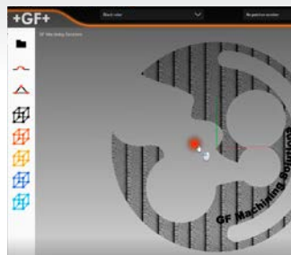
Perlage decoration toolpath, created with LaserCAM™
