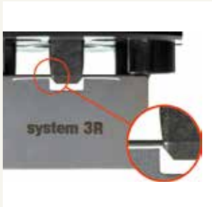
The lip edge of the pallet is angled to match the angle of the boss. This maximises the mating surface area between the parts, resulting in precision alignment, minimal wear and enduring precision.
